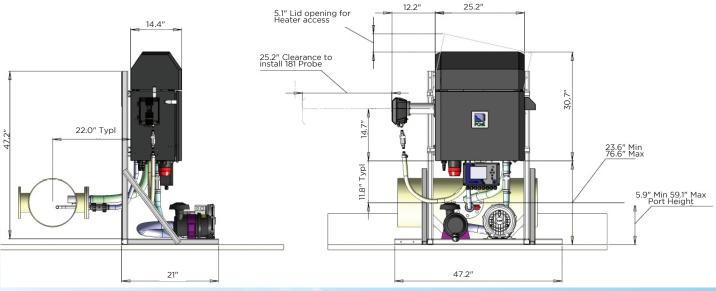
Analyzer unit to be located above and closely coupled to sampling probe
